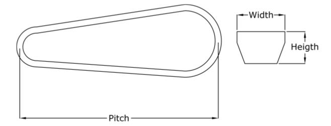
$\begin{array}{ll} \text{Datum Llength} = 6895 \\ \text{Height} & = 10 \\ \text{Length inside} & = 6870 \\ \text{Type} & = BB270 \\ \text{Width} & = 17 \end{array}$
